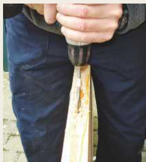
▲ Pic.2 Using a flat bit in the cordless drill to cut the mortise...
